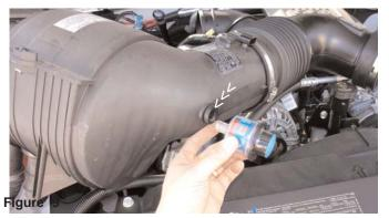
Pull the air restrictor gauge from the stock grommet as shown above.
