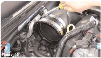
The new step hose is inserted over the turbo inlet tube. Two clamps are placed over the step hose. The clamp that is over the the turbo inlet tube is tightened at this point.
