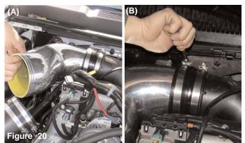
Once you have aligned the cast intake to the step hose, continue to press the intake into the hose (A) The power-band on the intake side is semi-tightened to hold the intake in place (B).
