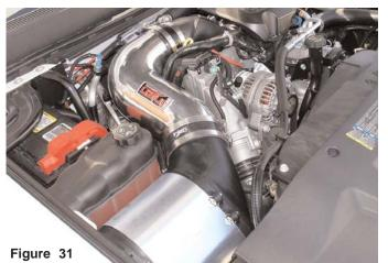
Check the entire system for the best possible fit. Once you have checked the entire system for leaks, rubbing or rattling, continue to tighten all nuts, bolts and clamps. Reconnect the negative battery terminal prior to starting the engine.
