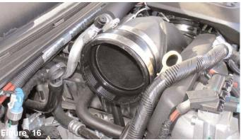
The new step hose is now installed over the turbo inlet tube.
