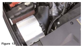
The new performance air box should be sitting flush in the grommets and the plenum should be facing in the direction of the turbo inlet tube.
