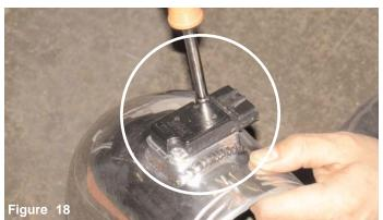
Use the m4 x 10mm button head bolts in this kit to fasten the mass air flow sensor to the machined sensor adapter. A 2.5mm allen
