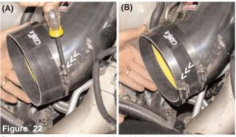
Place one power-bands over the 5 1/2" straight hose and tighten the clamp to prevent the hose from slipping off (A). Place the remaining power-band over the opposite end of the 5 1/2" straight hose but do not tighten this clamp at this point (B).
