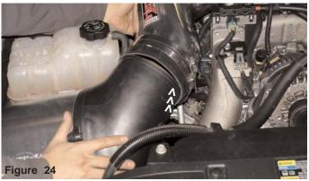
Once you have installed the straight hose over the end of the intake, continue to press the hose over the intake plenum.
