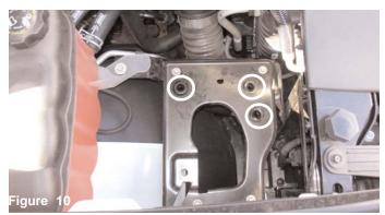
The pegs on the air box mounting plate are designed to be inserted into the three stock grommets that are circled above.
