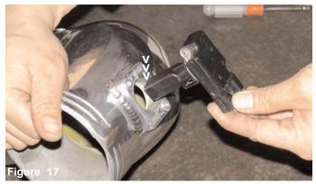
The mass air flow sensor is pressed into the machined sensor housing located on the cast intake. Rub a small amount of light oil around the O-ring to prevent the O-ring from kinking up in the sensor opening.
