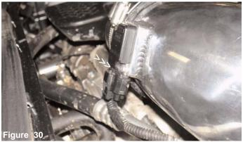
The electrical harness clip and mass air flow sensor are now properly connected.
