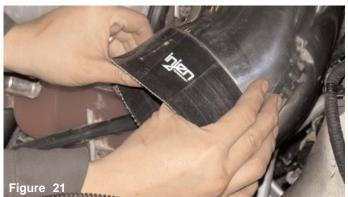
The 5 1/2" straight hose is slipped over the end of the cast intake. Press the straight hose no more than 1" or half the length of the straight hose.
