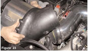
The air box is lifted in order to align the air box plenum to the cast air intake straight hose.
