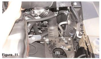
The pegs on air box mounting plate (A) are designed to be pressed into the stock grommets for easy installation (B).
