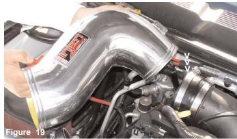
The cast intake is lowered and aligned with the step hose over the turbo inlet.
