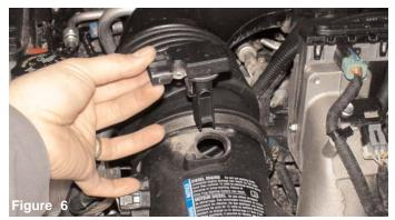
Once you have removed the bolts, continue to pull the mass air flow sensor out of the sensor housing.
