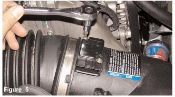
Use the T20 torx bit to loosen and remove the bolts on the mass air flow sensor.
