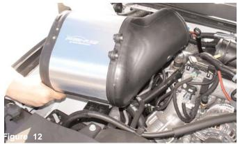
The Injen/AMSOIL air box should now be aligned over the stock grommets then lowered into the grommets.
