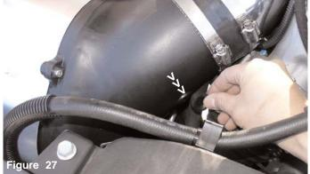
Press the Injen/AMSOIL grommet into the the 3/4" pre-drilled hole located on the plenum. Note: The grommet has been designed to be rotated for proper clearance of the air restrictor gauge.
