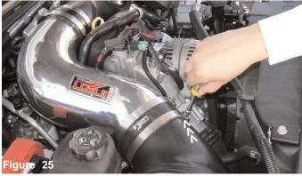
Once you have inserted the cast air intake into the air plenum, continue to adjust the power band for best fit, then begin to tighten clamp. Page 4 of part# PF7075
