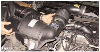
Once all clamps and hoses have been removed from the air box cleaner, continue to pull the entire air box out of the engine compartment. Pull up on the air box to disengage air box pegs from the grommets.
