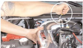
Tighten the clamp on the turbo inlet side once you have adjusted the cast intake.
