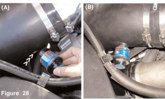
The stock air restrictor gauge is now pressed into the Injen/AMSOIL grommet t(A). Once you have inserted the restrictor gauge into the grommet, continue to rotate grommet and restrictor gauge until you have found the best position (B).
