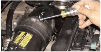
Loosen clamp on the turbo inlet tube connected to the air intake duct.
