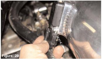
Reconnect the electrical sensor clip to the mass air flow sensor. Press the harness clip over the mass air flow sensor until you hear them snap together.
