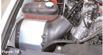
Another view of the Power air plenum designed to direct and speed up air flow. The new performance air box should be sitting flush in the grommets and the plenum should be facing in the direction of the turbo inlet tube.
