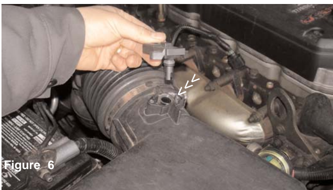
Figure 4 Depress the tab on the electrical harness clip and disengage it from the mass air flow sensor as shown above.
