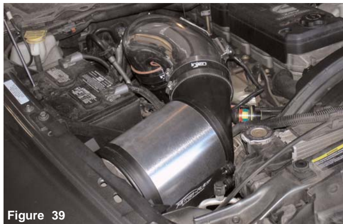
Figure 37 The air restrictor gauge is now sitting flush over the grommet. Rotate the grommet and restrictor gauge until you have positioned it for best possible fit, away from any lines.
