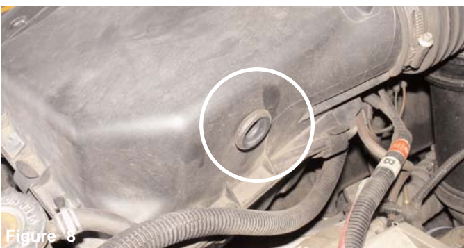
Figure 6 Once you have removed the screws from the MAFS, continue to pull the MAFS out of the sensor housing.
